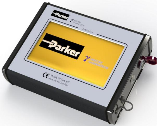
**AshGraffix, together with the Ash-Probe, is a portable instrument for accurately measuring the ash content of piles, wagons or trucks of coal in real time.**
