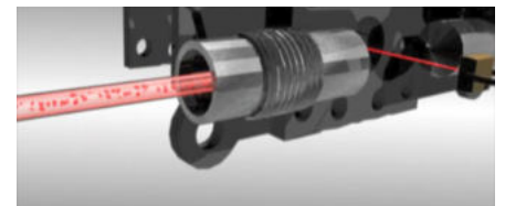
Fig 1. In simple terms a controlled column of contaminated fluid enters the laser optical scanner chamber. This design maintains contamination distribution within the fluid.
